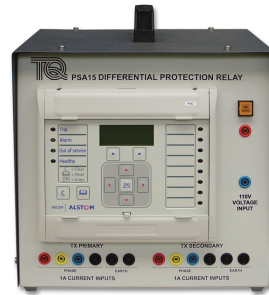
DIFFERENTIAL PROTECTION RELAY (PSA15)
